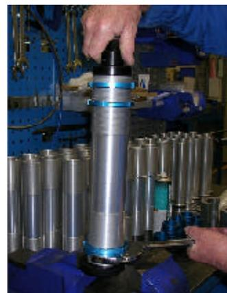
3. Remove from the vice and fit the Cap Clamp (Tool 2) to the knurled Airjack Cap. Locate the Air Jack and Cap Clamp vertically, clamping the Cap Clamp in the vice. **(See Fig 2.)**
