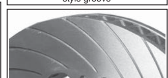
CR4, CR8, CR12 & CR24 = Curved Grooves. (Backward facing running out on O/D to clear debris. Only used on thick wall discs). The number specifies grooves per face.
