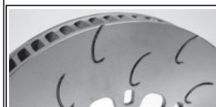
RA = 'J' Hook Design. Gives improved bite and debris clearance and reduces distortion / vibration, outer grooves run out to O/D. Thick wall discs only
