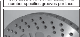
D & SD = Cross Drilled. (Drilled holes chamfered). Still preferred with some pad materials but can compromise disc life.
