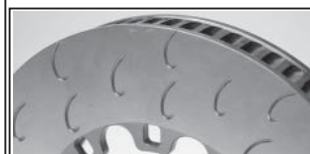
RC = 'J' Hook Design. As RA design but with 3 hooks across face. This design gives improved bite and debris clearance and reduces distortion / vibration. Thick wall discs only
