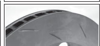
PG = Partial Groove. Shorter length groove pattern
