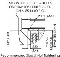
Recommended Stud & Nut Tightening Torque = 22Nm (16lb/ft)
