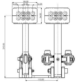
SETING UP THE BALANCE BAR ADJUST THE PUSHRODS SO THAT THE BALANCE BAR ISPERPENDICULAR TO THE PUSHRODS UNDER MAXIMUM LOAD, THE SYSTEM IS THEN SQUARE. IT IS NOT IMPORTANT THAT THE SYSTEM IS SQUARE WHEN RELEASED, BUT IT HAS TO BE UNDER LOAD.
