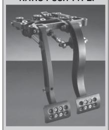
This multi ratio push type pedal box allows the pushrod to remain straight, eliminating all side loads therefore making it very efficient. The master cylinders connect directly to a high efficiency balance bar.
