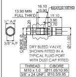
THREADED OUTLET & 1 WAY VALVE FITTED CP6300-32 BLEED COUPLING WITH NON-THREADED OUTLET & 1 WAY VALVE FITTED
