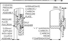
EFFECT WILL DETERIORATE AND COMPONENTS SHOULD BE SERVICED WITH THE ABOVE KIT WHEN EITHER THE BELLEVILLES BECOME LOOSE OR WHEN DIMENSION 'X' FALLS BELOW 1.00.TAKEN AS THE AVERAGE OF 4 EQUALLY SPACED MEASUREMENTS AROUND THE CIRCUMFERENCE OF THE BELLEVILLE.
