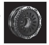
In 2016 AP Racing launched a range of Ø140 & Ø184mm clutches "PRO To < que". These new Radi-CAL<sup>TM</sup> styled assemblies offer all the usual carbon clutch benefits, such has long life, durable and abuse resistant, improved modulation and most significant a more affordable carbon clutch solution for all forms of motorsport.
