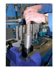
**3.** Once the Bearing housing is unscrewed completely from the Body, the Air Jack Piston Assembly can be withdrawn from the Body in one piece. **(See Fig 2.)**
